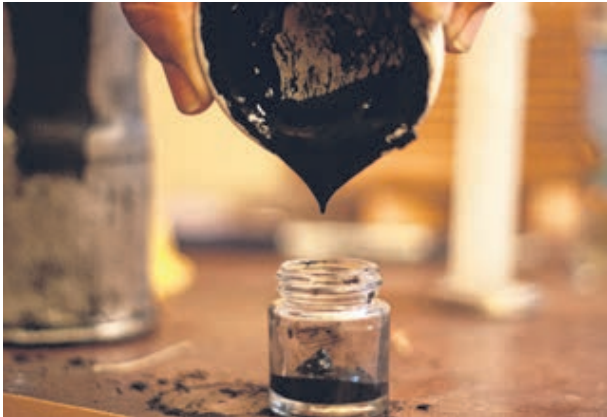
Kaalink is attached to a vehicle's tail pipe to filter out residual soot (far left). This is then chemically processed and turned into a purified carbon pigment that, in turn, becomes Air-Ink (left), which was used to paint this mural in Hong Kong (below). PHOTOS: GRAVITY LABS, TIGER BEER
