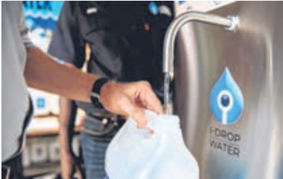
I-Drop's water-purification system uses a nanocarbon configuration to filter out viruses, bacteria and cysts – anything that is carbon-based and could make someone sick – while retaining the water's minerals. PHOTO: CHIVAS THE VENTURE
