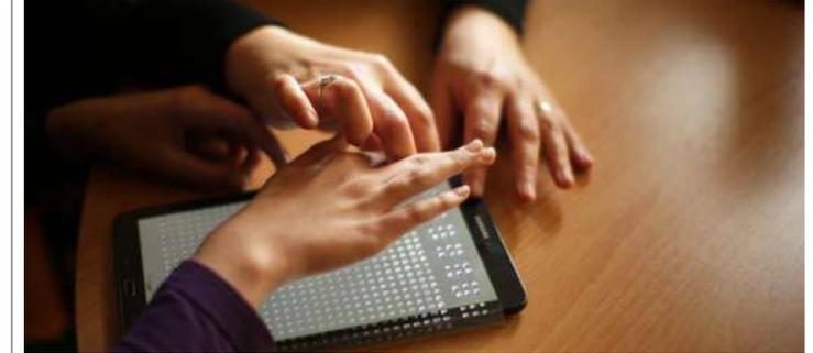
The device consists of a tablet, a relief grid placed over the screen, and an application.
